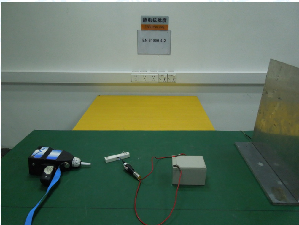
Photo 2 Electrostatic discharge Test Setup
