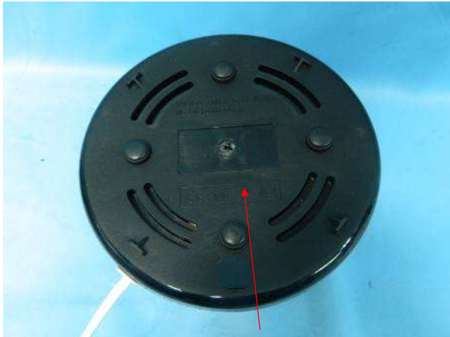
Marking label position on bottom enclosure
