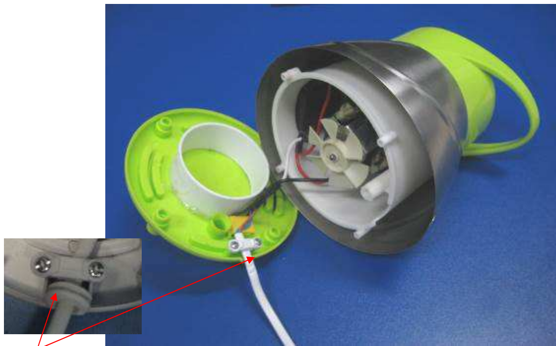
Bushing Internal view of model KL-217G and KL-217E
