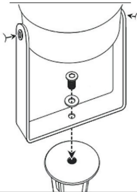
2. Use the same hex screw and washer to fix the holder of the spotlight to the stake. Be aware that you fix it tightly so the spotlight will not shake.
