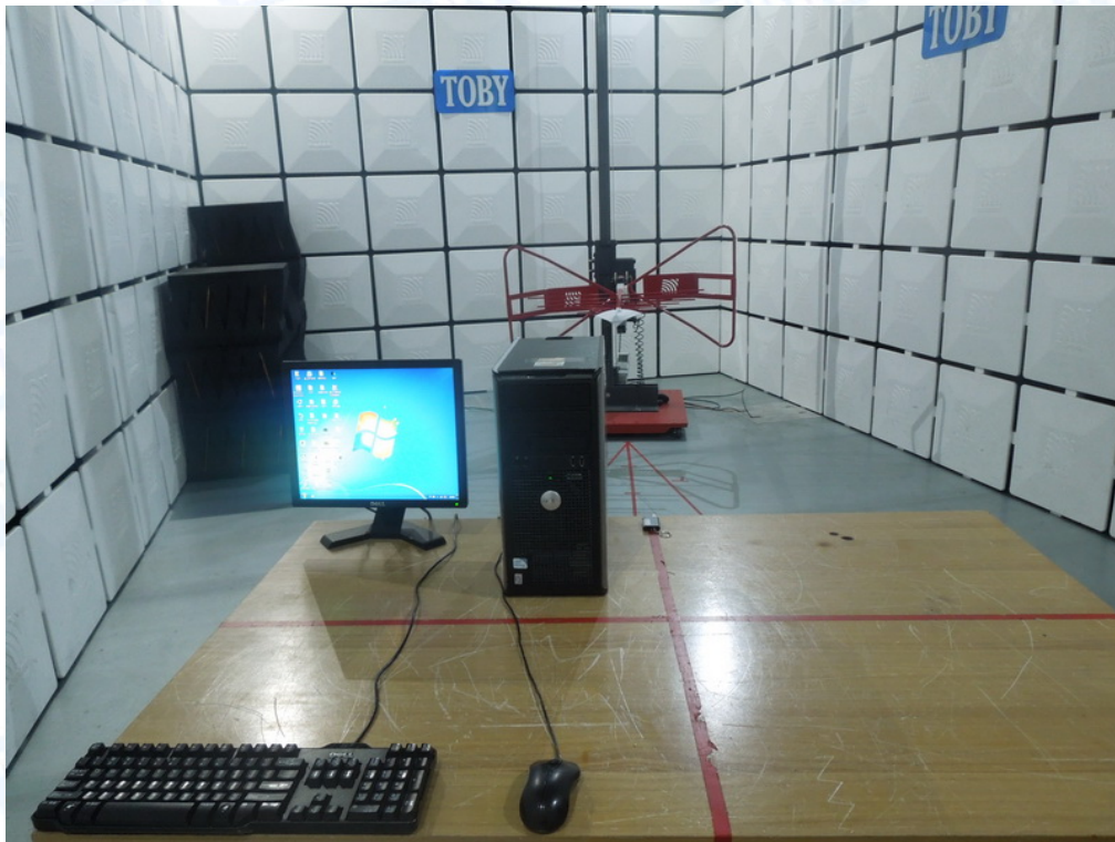
Photo 2 Radiated Emission Test Setup
