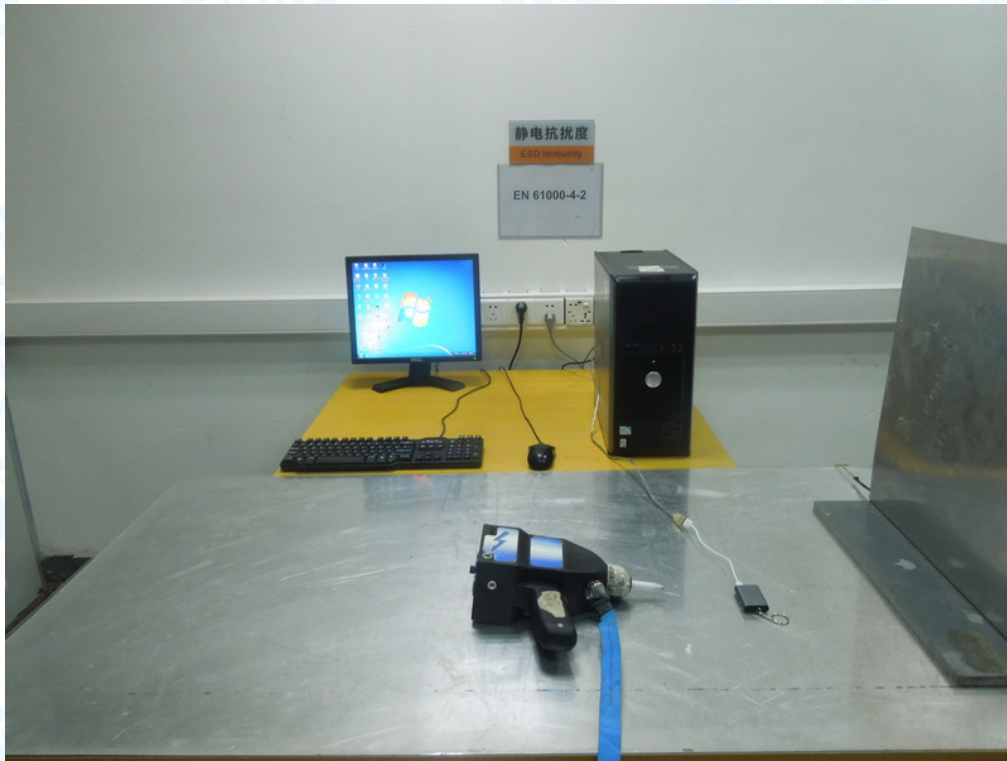
Photo 4 Electrostatic Discharge Test Setup
