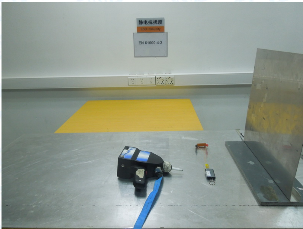
Photo 4 Electrostatic Discharge Test Setup
