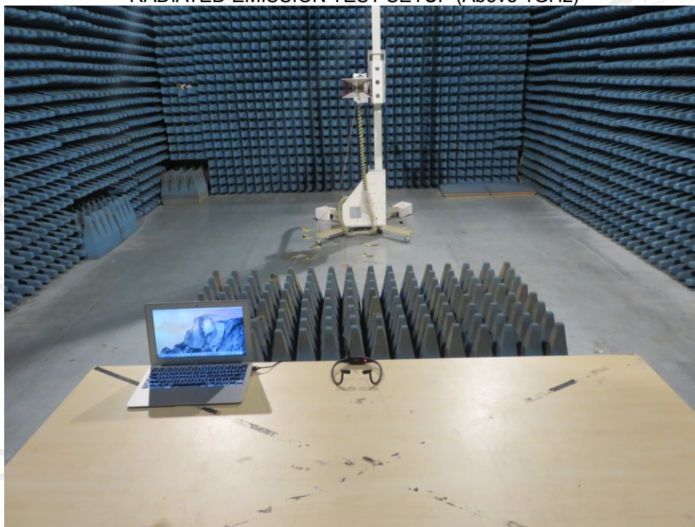
RADIATED EMISSION TEST SETUP (Above 1GHz)
