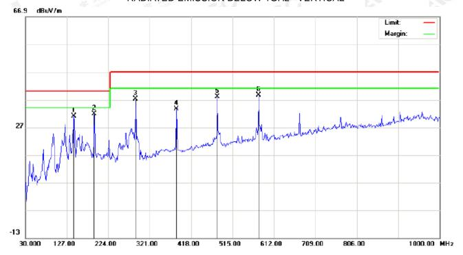
Site: site #1 Polarization: Vertical Temperature: 22.4 Limit: EN55032 ClassB 3M Radiation Power: Humidity: 52.5 %
