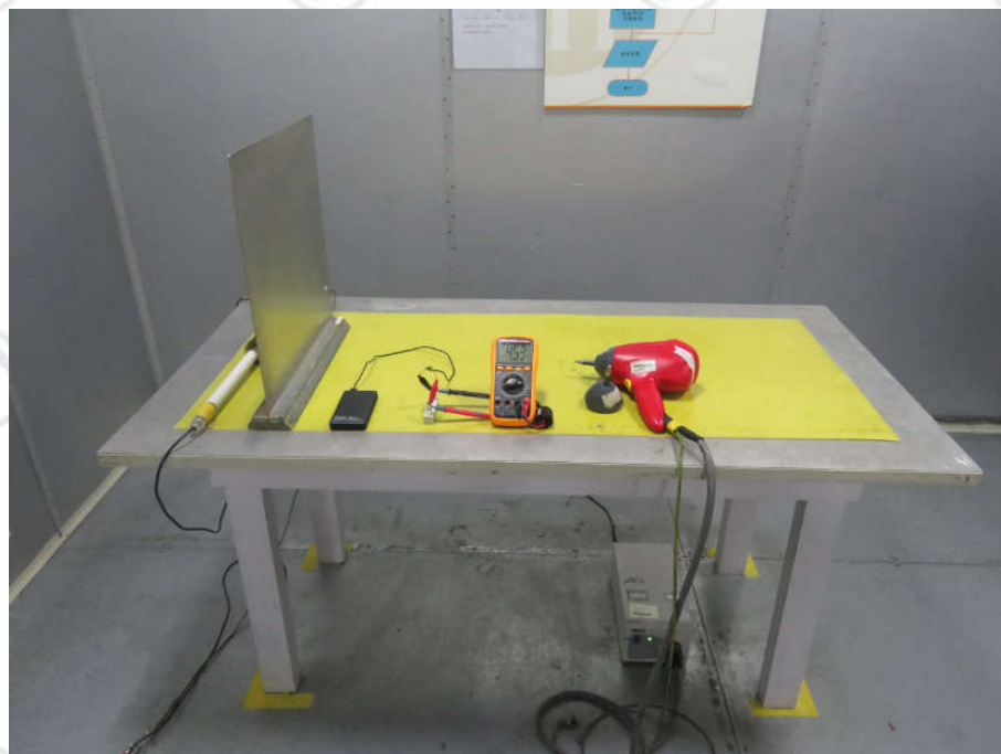
ELECTROSTATIC DISCHARGE TEST SETUP
