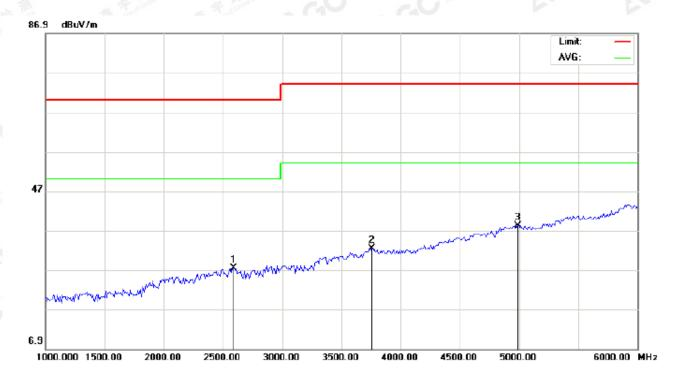
Site: site #1 Temperature: 24.6 Polarization: Vertical Limit: EN55032 Class B Above 1G(Peak) Humidity: 54.6 % Power:
