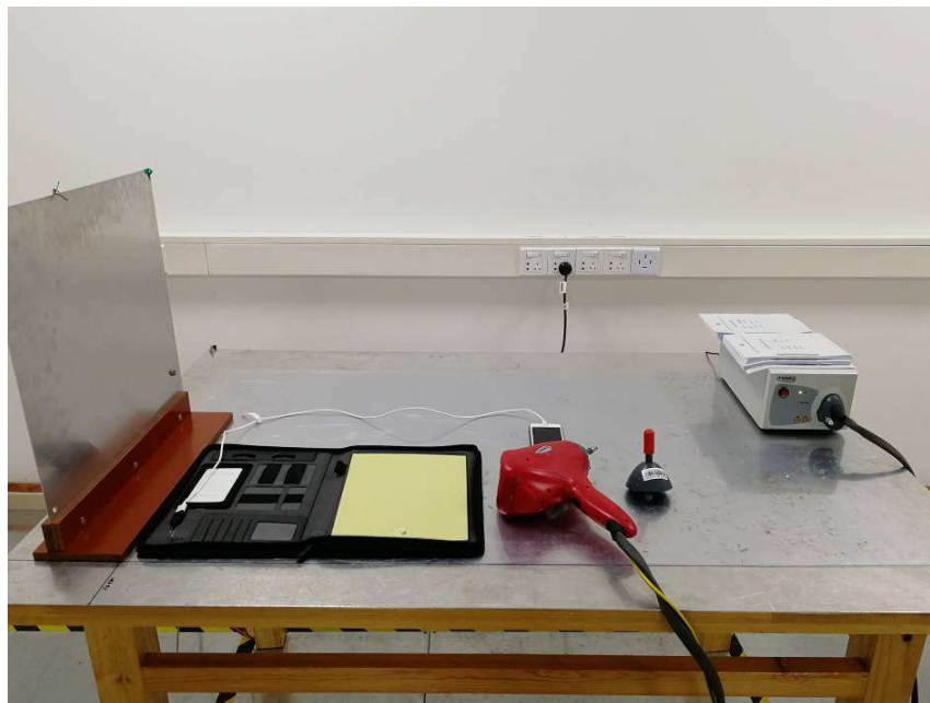
Set-up for Electrostatic discharge immunity (ESD)
