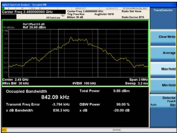
20dB Bandwidth plot on channel 78 (1Mbps)
