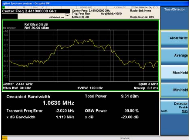
20dB Bandwidth plot on channel 78 (2Mbps)
