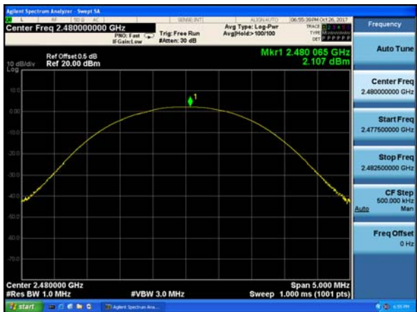
Peak output Power plot on channel 78 (3Mbps)
