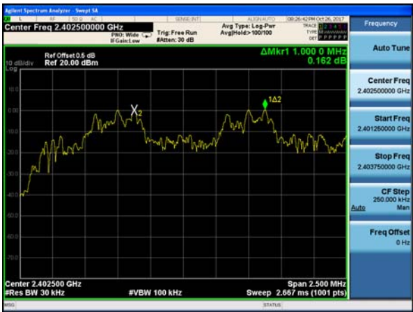
(3Mbps) Channel Separation plot on channel 39-40
