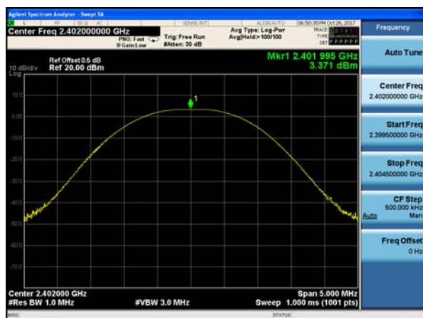
Peak output Power plot on channel 39 (1Mbps)
