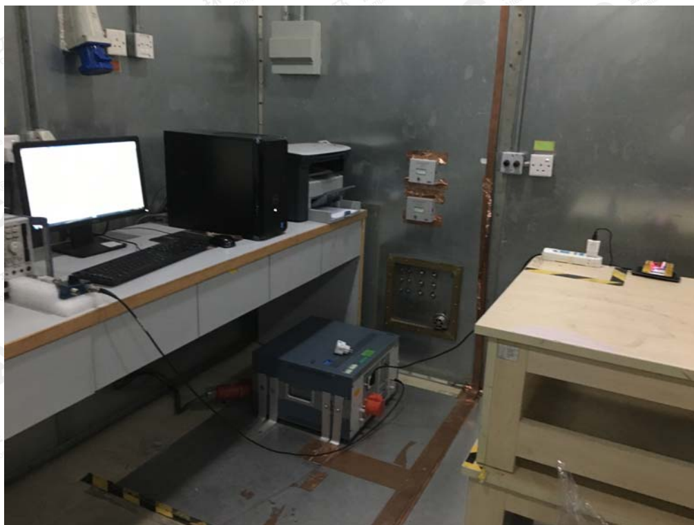
RADIATED EMISSION TEST SETUP
