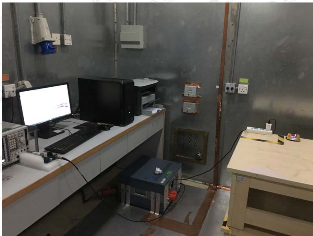
RADIATED EMISSION TEST SETUP
