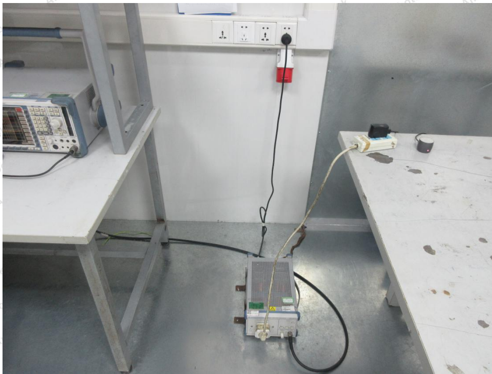
Photo of Conducted Emission Test
