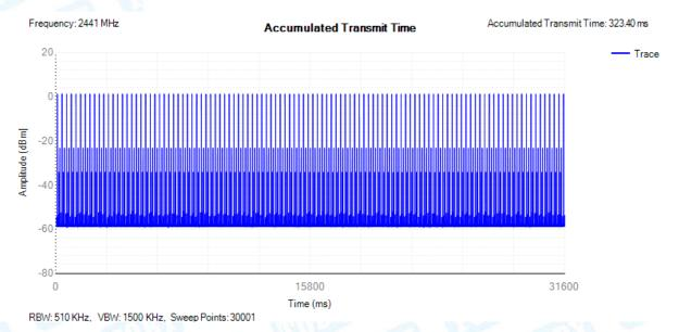
**Accumulated** Frequency **Measure Time Dwell Time** Limit (ms) **Burst Number** Result Mode (MHz) (ms) (ms) 110 **PASS** 2441 **3DH5** <=400 31600 323.4
