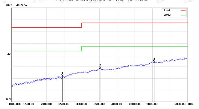
Site: site #1 Polarization: Vertical Temperature: 24.6 Limit: EN55032 Class B Above 1G(Peak) Power: Humidity: 54.6 %
