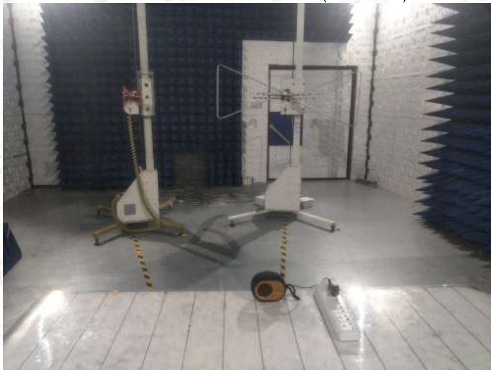
RADIATED EMISSION TEST SETUP (Above 1GHz)
