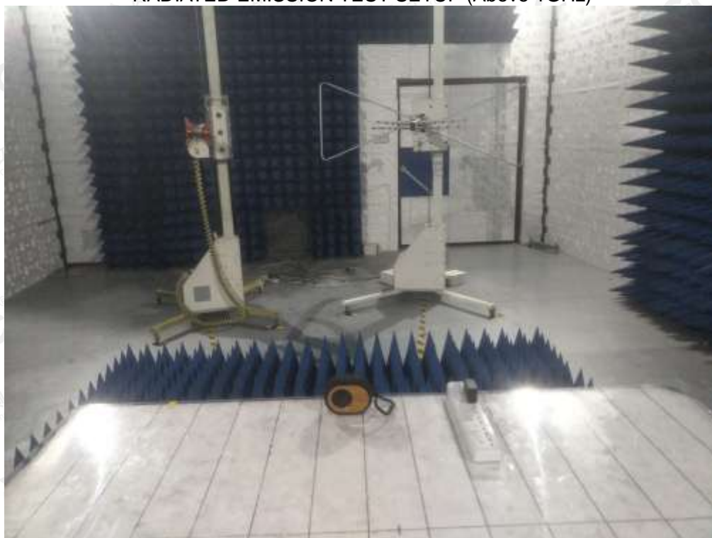
RADIATED EMISSION TEST SETUP (Above 1GHz)
