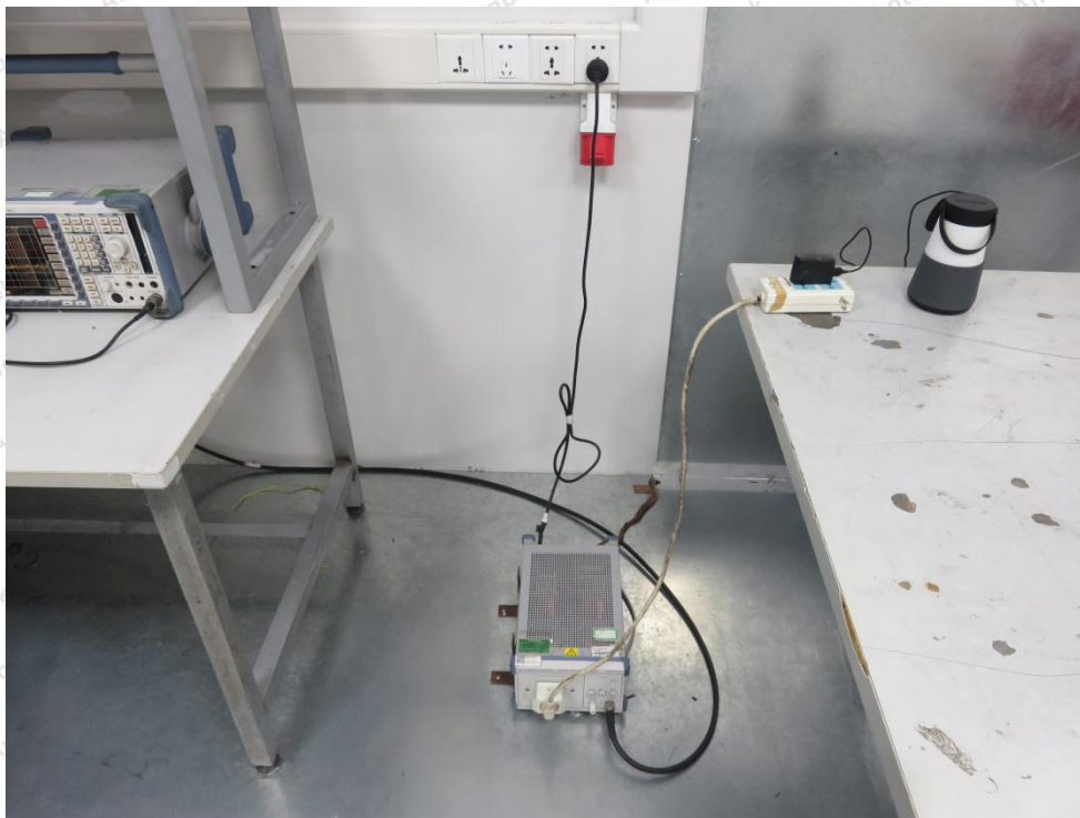
Photo of Conducted Emission Test
