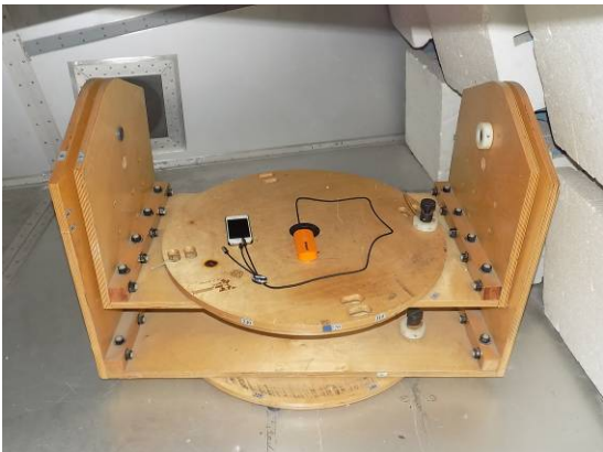
7.3. Photo of RF field strength Immunity measurement (R.S.)
