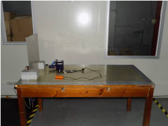
7.3. Photo of RF field strength Immunity measurement (R.S.)
