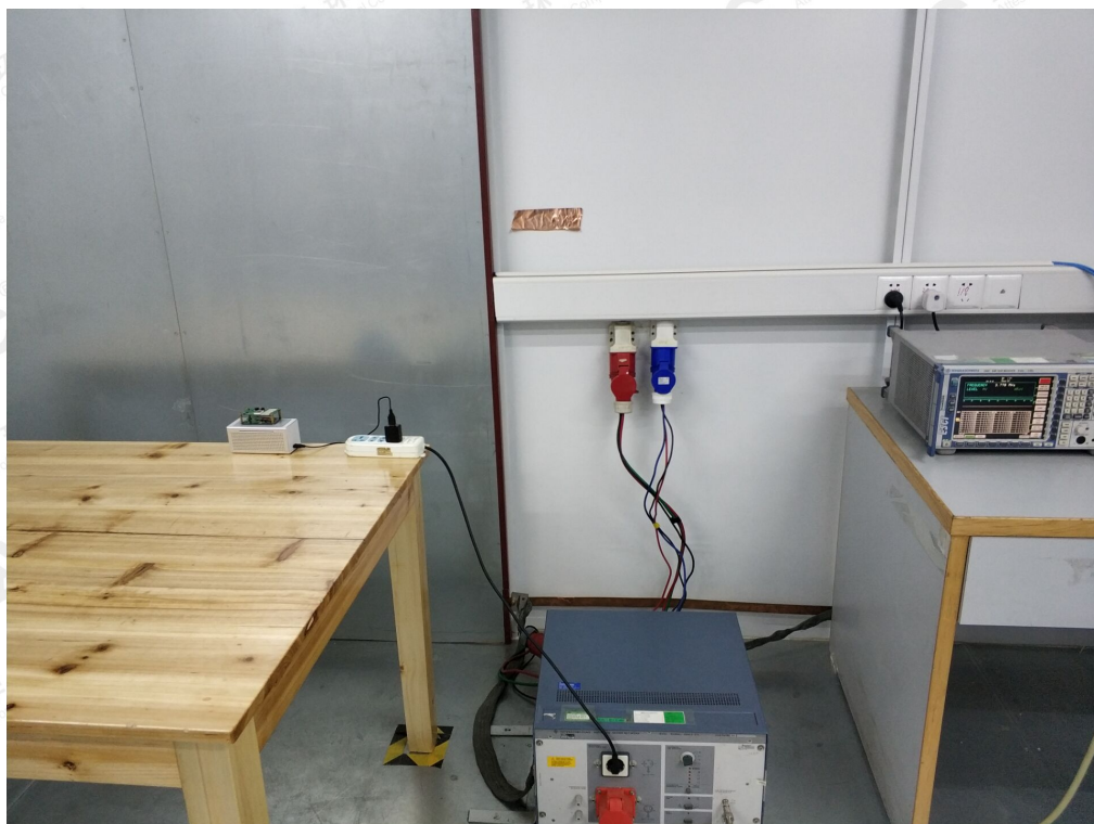
RADIATED EMISSION TEST SETUP
