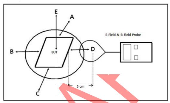
Note: Position A: Front of EUT; Position B: Left of EUT; Position C: back of EUT; Position D: Right of EUT; Position E: Top of EUT
