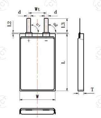
T: 9.50mm Max W:55.0mm Max L:65.50mm Max Cell (Unit: mm)
