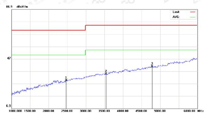
Site: site #1 Limit: EN55032 Class B Above 1G(Peak) Polarization: Horizontal Power:
