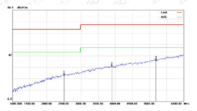
Site: site #1 Polarization: Vertical Temperature: 24.6 Limit: EN55032 Class B Above 1G(Peak) Power: Humidity: 54.6 %
