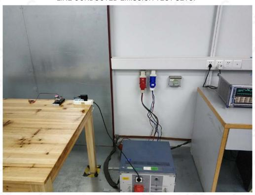
RADIATED EMISSION TEST SETUP
