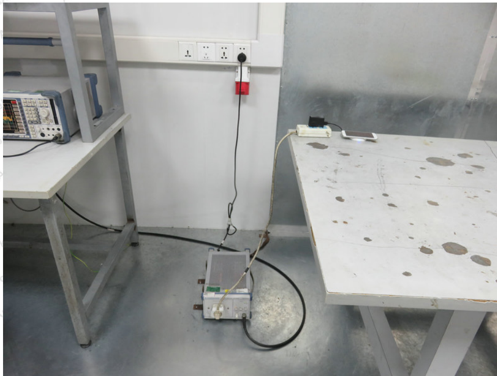
Photo of Conducted Emission Test
