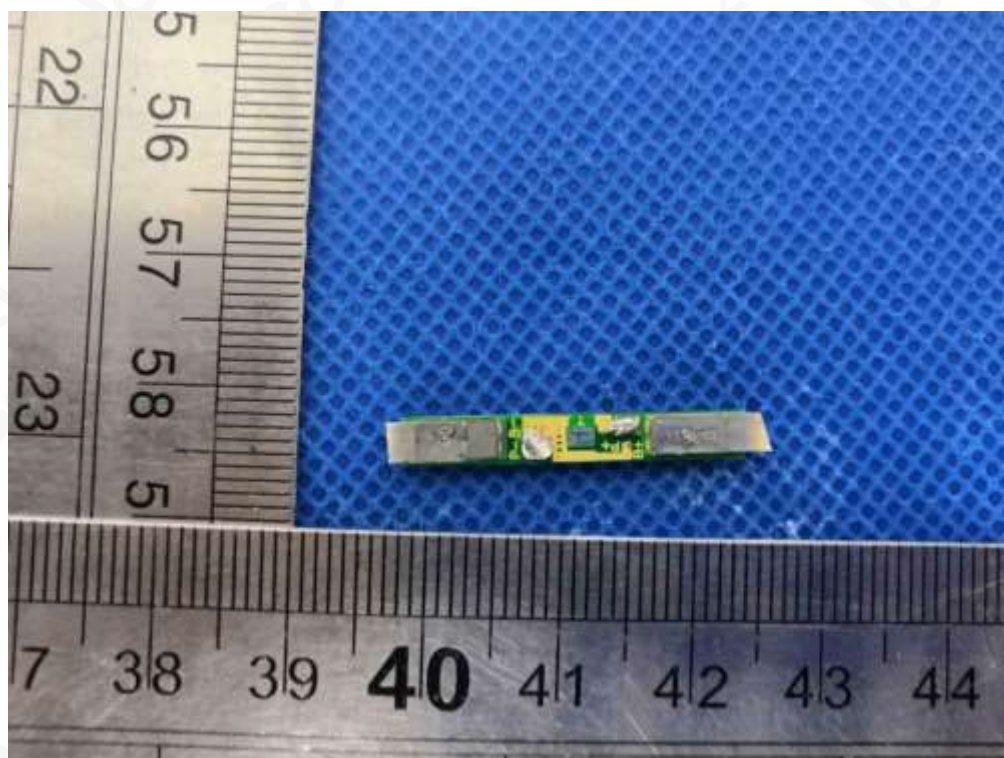
Fig.9 – Battery protection circuit
