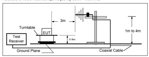
Radiated emission test set-up, frequency above 1000MHz
