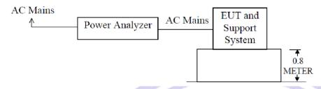
This test was performed as per EMC Basic Standard EN61000-3-2
