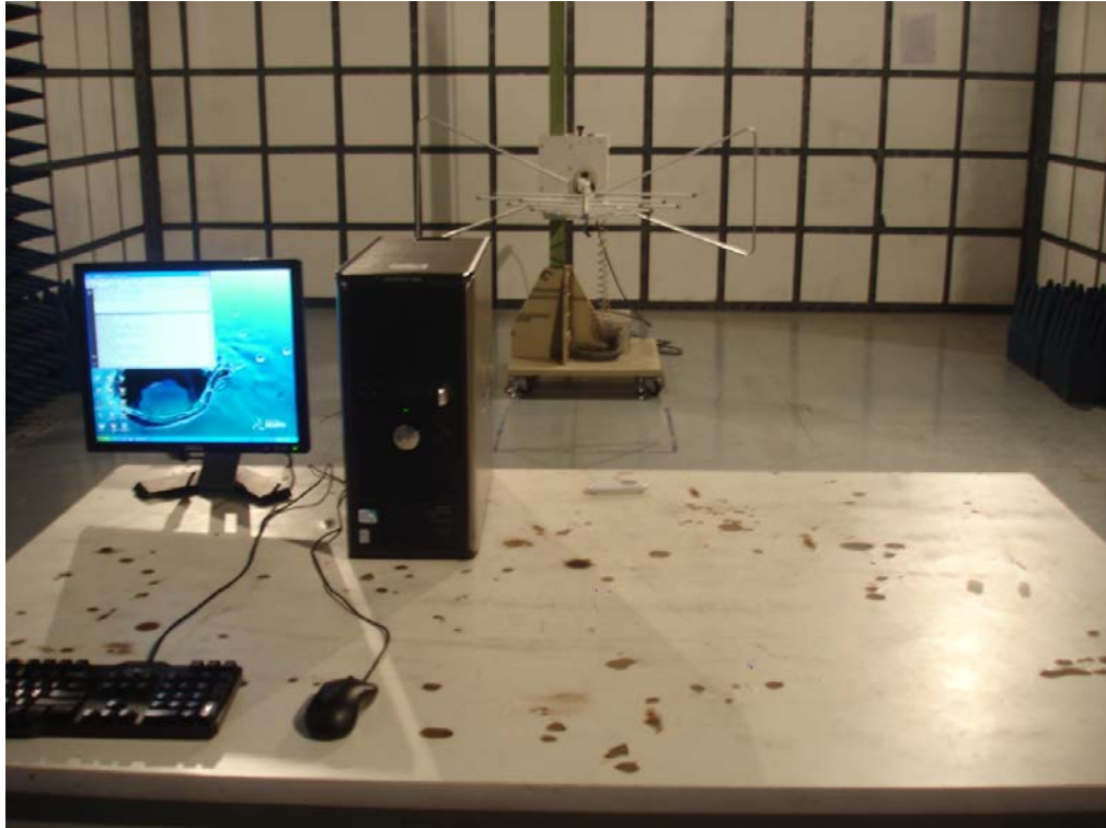
Photo 2 Electrostatic Discharge Test Setup
