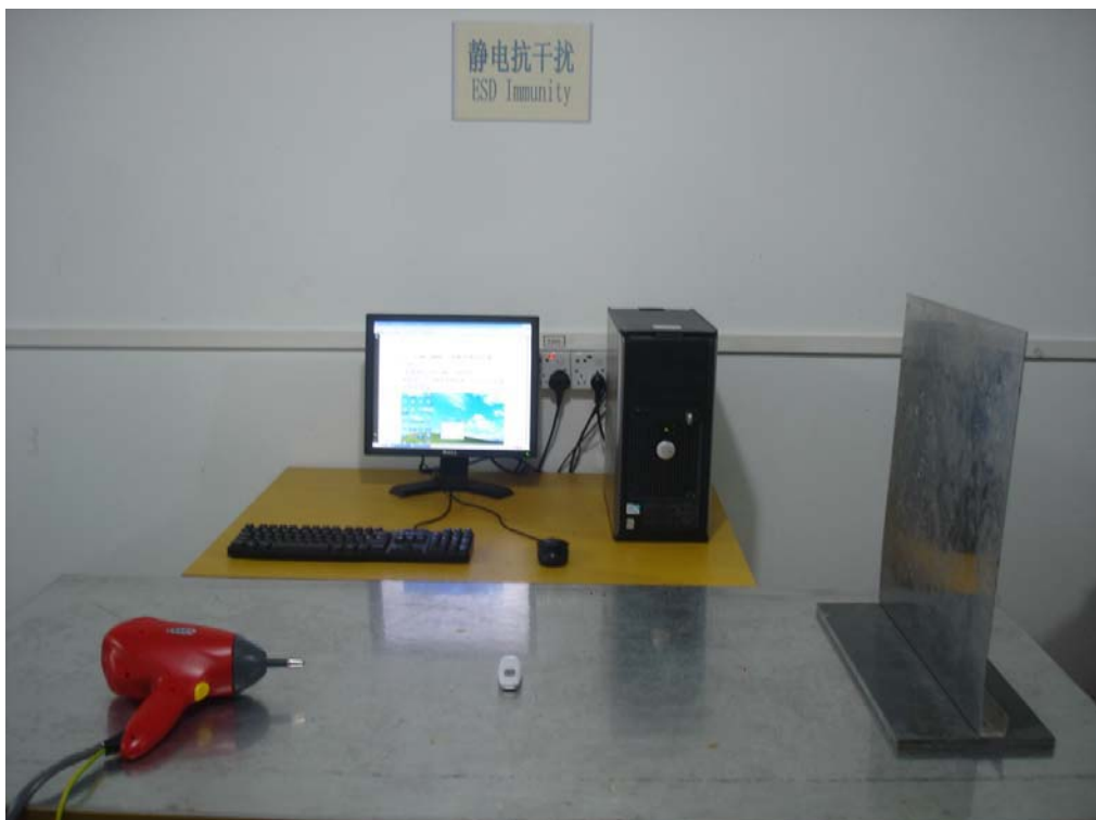
Photo 2 Electrostatic Discharge Test Setup
